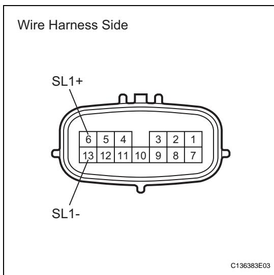
(a) Disconnect the B32 wire connector.
